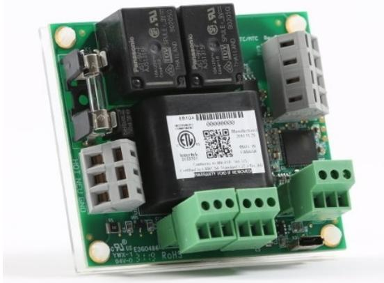
Embedia's Solarai™ EB1 GROUP is a BACnet MS/TP device capable of independent or grouped control for one motorized system. It is designed for response based automation and out-of-the-box low voltage control of roller shades, venetian blinds, operable louvers, and other devices using any standard 4-wire AC motor.
