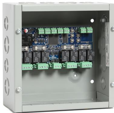
Embedia's Solarai™ EB4 GROUP is a BACnet MS/TP device capable of independent or grouped control for four motorized systems. It is designed for response based automation and out-of-the-box low voltage control of roller shades, venetian blinds, operable louvers, and other devices using any standard 4-wire AC motor.
