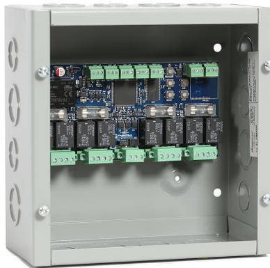
Embedia's Solarai™ EB4 Plus is a BACnet MS/TP device capable of advanced independent or grouped control for up to four motorized systems. It is designed for unrivalled intelligence with predictive environmental control of roller shades, venetian blinds, operable louvers, and other devices using any standard 4-wire AC motor.
