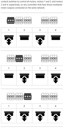
Closing a contact momentarily will start the motors moving in the corresponding direction. Closing both contacts will stop the motors.
