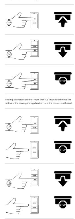
The onboard contact closure (dry contact) input(s) can be reconfigured to control any number of motors on the connected network using the Embedia InSight App (free download) in conjunction with the USBIF-WiFi Add-on (sold separately) plugged into the onboard USB port of any controller on the connected network. Contacts can also be regrouped to provide more advanced functionality like scenes.
